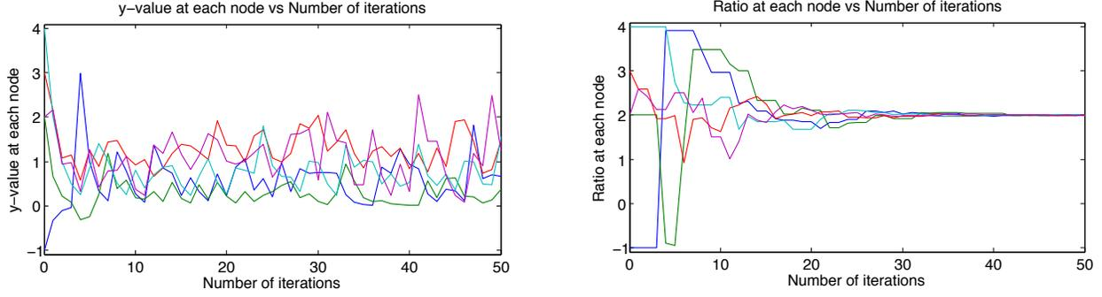
Fig. 2. The update formula in (7) for the network on the left of Figure 1 with weights  $P$  and  $y[0] = y_0$ , does not converge (left); however, if we run ratio consensus in (7) and (8) with initial conditions  $y[0] = y_0$  and  $z[0] = \mathbf{1}$  respectively, then average consensus is asymptotically reached for the ratio  $y_j[k]/z_j[k]$  (right).
