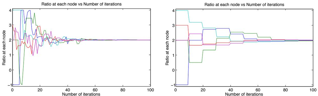
Fig. 4. Comparison of convergence time for running ratio consensus in (7) and (8) for uniformly random delays between 0 and 10 (equiprobable as before), and for updating every  $\bar{\tau} = 10$  so that all the delayed information is collected.
