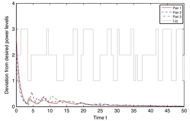
**Fig. 1.** Simulation of the switched network represented by matrices  $\mathbf{C}_1, \mathbf{C}_2$  and  $\mathbf{C}_3$ , each consisting of three communication pairs. The plot shows the evolution of the deviation from the desired power levels; the switching sequence  $\sigma(t)$  is also shown (that is,  $\sigma(t) = 1$  means the network is represented by matrix  $\mathbf{C}_1$ , and so on).
