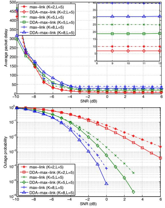
Fig. 6. Average delay (top) and outage probability (bottom) for the DDA – max – link algorithm for  $K = 2, 5, 8$  and  $L = 5$ .
