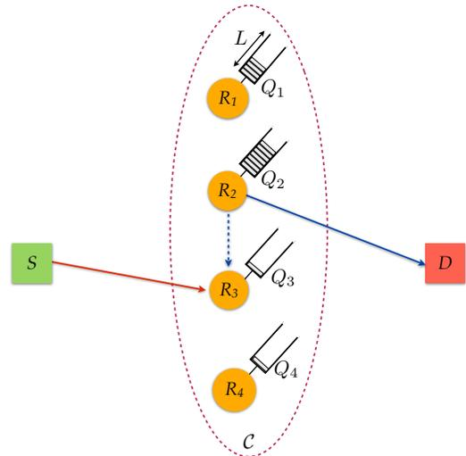
Fig. 1. A simple relay network that exemplifies the system model: Source  $S$  communicates with Destination  $D$  via a cluster of 4 relays  $R_k \in \mathcal{C}$ ,  $k \in [1, 4]$ .
