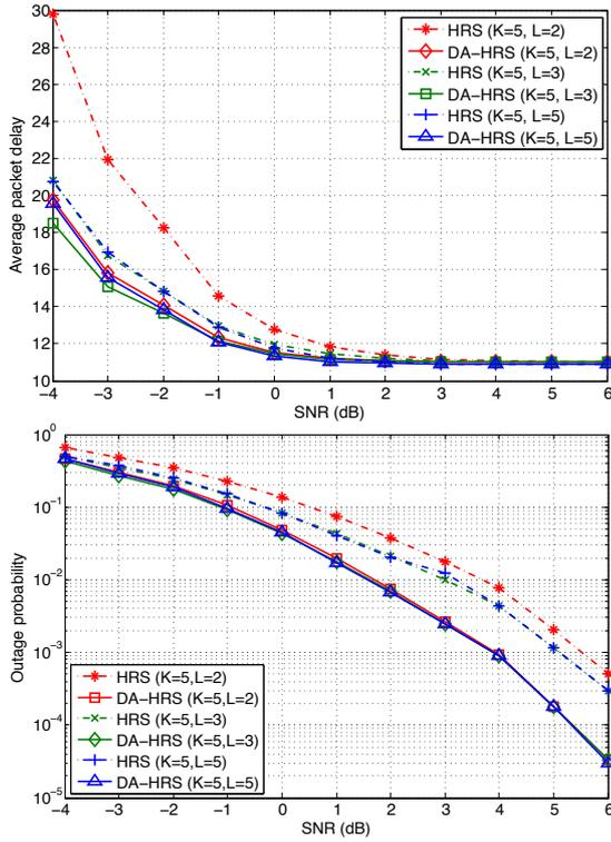
Fig. 3. Average delay (top) and outage probability (bottom) of DA – HRS for  $K = 5$  and  $L = 2, 3, 5$ .
