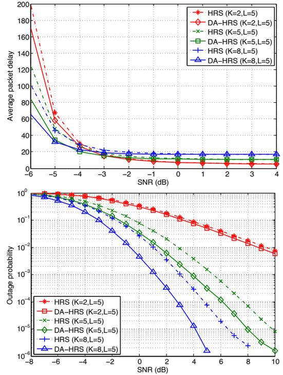
Fig. 4. Average delay (top) and outage probability (bottom) of DA – HRS for  $K = 2, 3, 4$  and  $L = 5$ .
