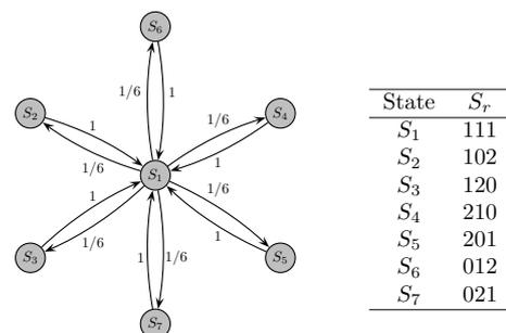
Fig. 2. DTMC of a network consisting of 3 relays at the high SNR regime, where the outage probability is negligible.
