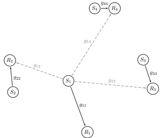
Fig. 2. Example of a wireless ad-hoc network of  $n = 8$  nodes, consisting of four communication pairs  $\{S_i \rightarrow R_i\}$ . The grey dotted arrows are included to indicatively show the interference caused to the receivers by  $S_1$ .
