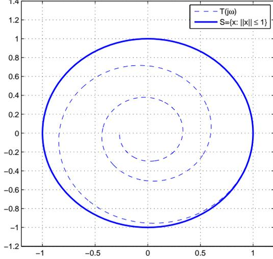
Fig. 1. The union of  $T(j\omega)$  is bounded by the unit ball. This is illustrated by an example in this figure for  $k_i = 2$  and  $T_i = 2$  ( $\left\{ \frac{2}{j\omega + 2} e^{-2j\omega} : \omega, \in \mathbb{R}_+ \right\} \subseteq S$ ).
