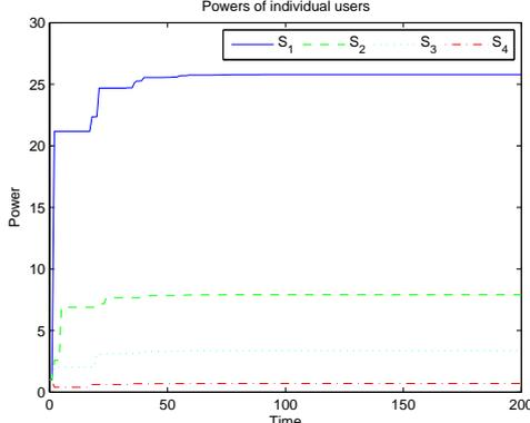
Fig. 3. Discrete-time FM algorithm with delays ( $T = \{15, 2, 17, 14\}$ ). The algorithm asymptotically converges to the desired SINR in a distributed manner.
